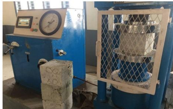
Fig: Cube placed in compressive testing machine
